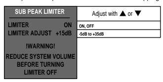
The MC-1 provides a Subwoofer Peak Limiter that prevents the subwoofer signal level from exceeding a preset value. The limit is factory preset to a level of +15dB. This setting can be changed within the limiter's operating range of -5dB to +35dB, with -5dB providing maximum limiting.
